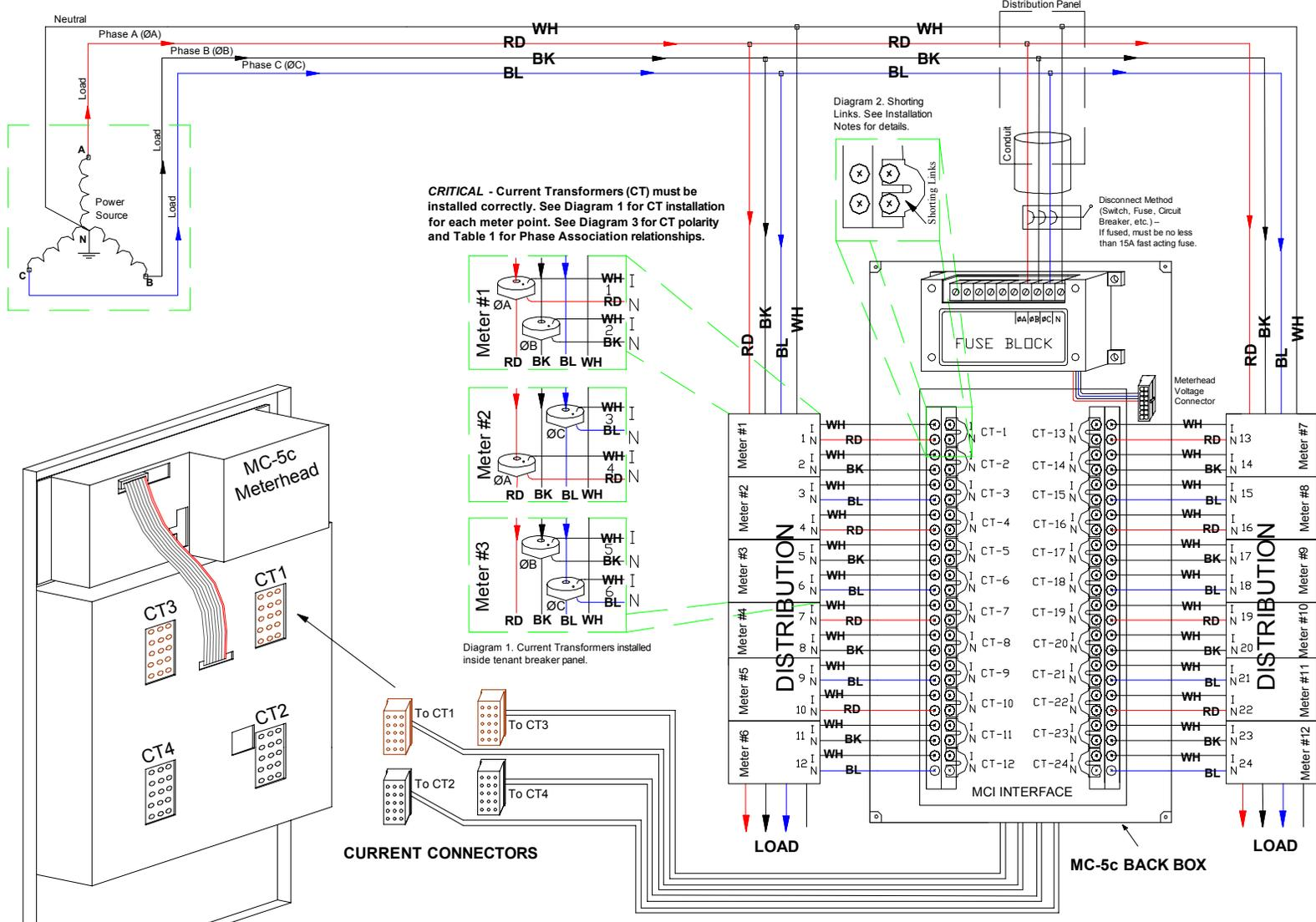
**CRITICAL - Current Transformers (CT) must be installed correctly. See Diagram 1 for CT installation for each meter point. See Diagram 3 for CT polarity and Table 1 for Phase Association relationships.**
