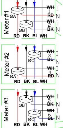
Diagram 1. Current Transformers installed inside tenant breaker panel.
